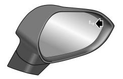
When there is a risk of collision, the warning lamp at the corresponding side illuminates. In this case, if the door opening action continues, the warning lamp will flash accompanied by an acoustic alarm.
