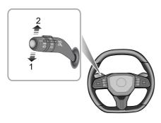
If briefly moved and released, the lever will reset immediately. The turn signal lamps and direction indicator lamps will flash three times and then go out.
