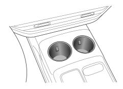
The centre console cup holder is located at the front end of the centre console armrest assembly and can hold cups or beverage bottles.
