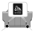
The Top-tether (as arrowed in the figure above) for auxiliary fixation of the child restraint is provided at the back of the rear seat backrest. The single top-tether of the child restraint must pass through space between the rods of the rear seat headrest and dual tether must pass from both sides of the rear seat headrest.
