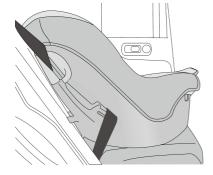
The child restraint can be secured to the rear seat by the lap and shoulder belts.
