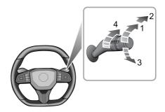
When the vehicle is powered on, operate the rotational switch to select different wipe speeds.
