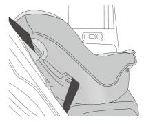
The child restraint can be secured to the rear seat by the lap and shoulder belts.
