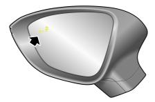
When there is a risk in reversing, the warning lamp at the corresponding side illuminates, and the instrument pack and entertainment display will show warning message. If the driver fails to take safety measures, the system will perform emergency braking.
