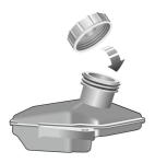
Note: Brake fluid will damage painted surfaces. If you accidentally spill the brake fluid on the painted surface, soak up any spillage with an absorbent cloth immediately and wash the area with water or car shampoo.
